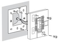
**10.** Attach the front module horizontally, making sure that each side of the front module fully aligns with that of the power unit, and then press each corner of the front module until you hear a click sound.
